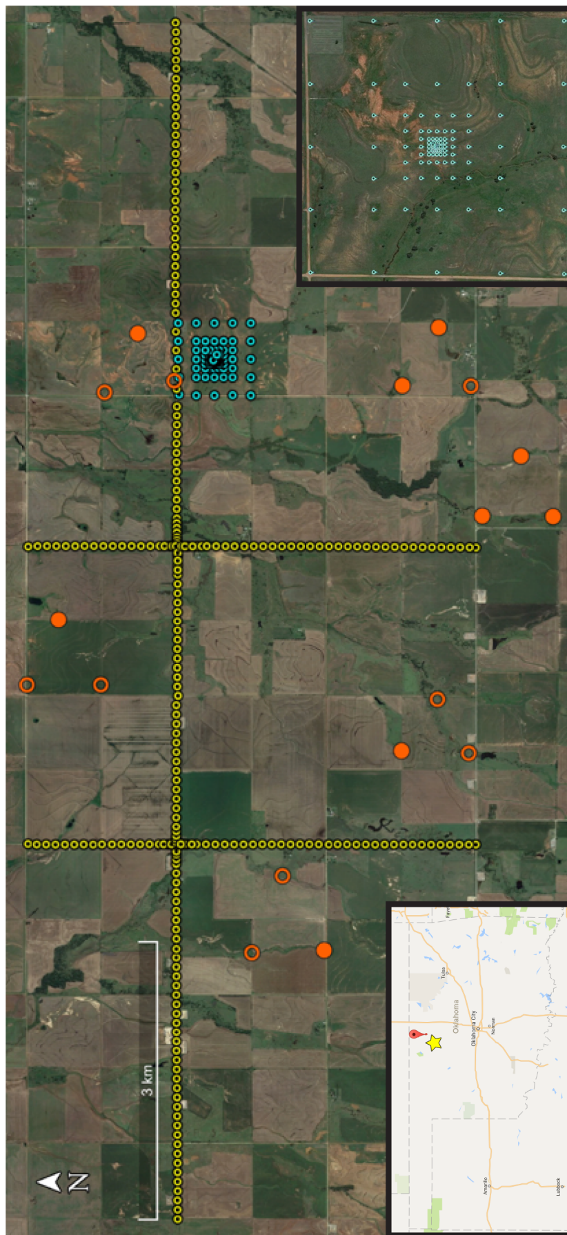
▲ Figure 1. Map of Wavefields Experiment in north-central Oklahoma. Nodes are denoted by large circles. Broadband stations are denoted by small circles. Solid large circles indicate the presence of co-located infrasound stations. Inset at the lower right is a zoomed-in view of the gradiometer array, whereas inset at the lower left shows the location of the deployment in Oklahoma (map marker) and Enid (star). The color version of this figure is available only in the electronic edition.
